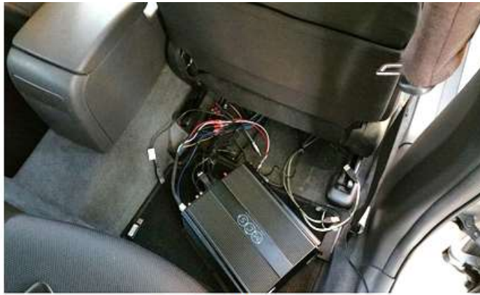
MCS Black Box Case pulled out from under the passengers seat
