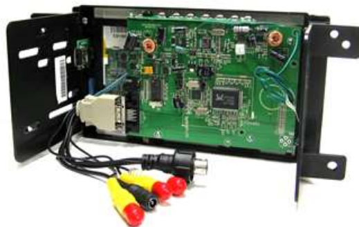
Rear circuit board of an EBY-701 7" touchscreen monitor in a double DIN housing
