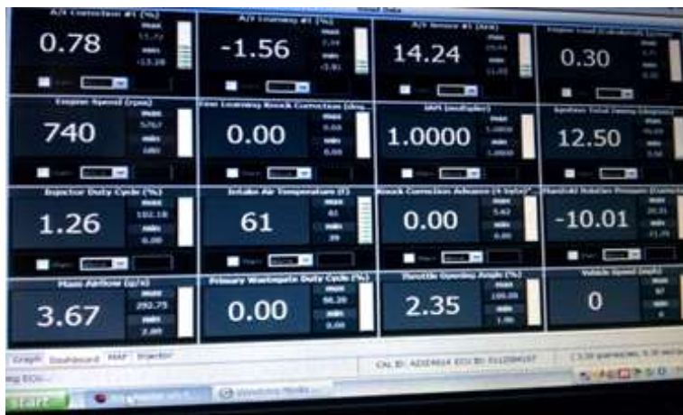
Older version of the RomRaider Dashboard on Windows XP showing real time output from the ECU
