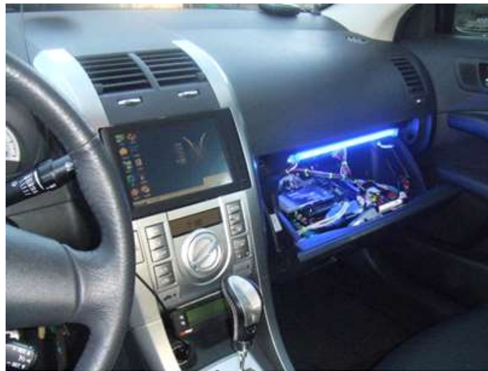
2005 Scion tC with a Car PC in the glove box
